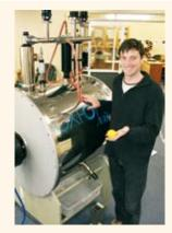
Riddet Centre researcher Dr Jason Hindmarsh stands alongside an MRI machine which he and Institute of Fundamental Sciences researcher Robin Dykstra have recommissioned. The machine will be used to track how the composition of a mix of milk and probiotic bacteria changes as it is dried and rehydrated.
