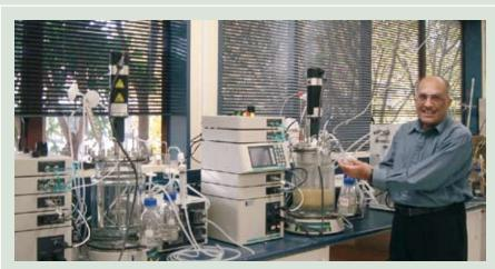
Professor Yusuf Chisti stands alongside two newly commissioned bioreactors. The bioreactors and their PC2-level containment facility complement recently-acquired equipment for recovering biological products. Professor Chisti is researching the use of biocatalysts – biotech microorganisms, animal and plant cells, enzymes, and subcellular components – to produce novel bioactive substances, vaccines, potential therapeutics, diagnostic antibodies and other high-value products.
